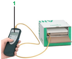
Configuring the drive in its packaging with the Multi-Loader tool VW3A8121
